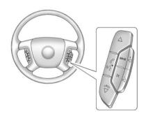
△ *I* ▽ : Press to change favorite radio stations, select tracks on a CD/DVD, or to navigate tracks or folders on an iPod® or USB device.
